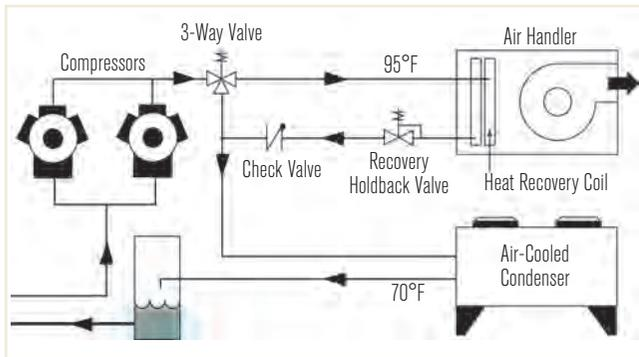
FIGURE 3 Condensing heat recovery system using air coil. Credit: *Advanced Energy Design Guide for Grocery Stores—Achieving 50% Energy Savings Toward a Net Zero Energy Building*
