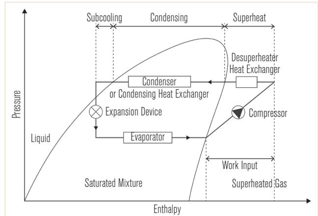
FIGURE 1 The refrigeration cycle showing condensing heat and superheat.
