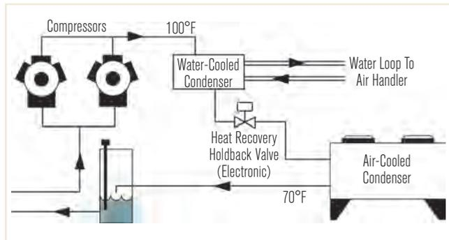
FIGURE 4 Condensing heat recovery using a water-cooled condenser. Credit: *Advanced Energy Design Guide for Grocery Stores—Achieving 50% Energy Savings Toward a Net Zero Energy Building*
